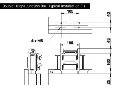
Box mounted along short face permitting up to seven 24-pin connectors to be mounted.
