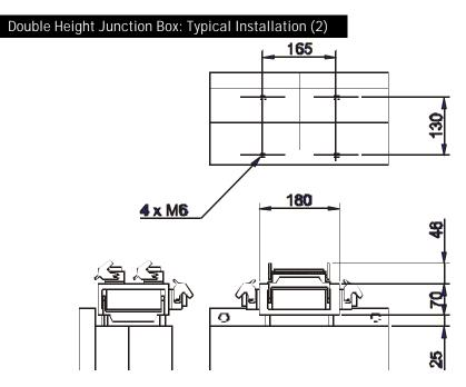
Box mounted along large face permitting up to six 24-pin connectors to be mounted.
